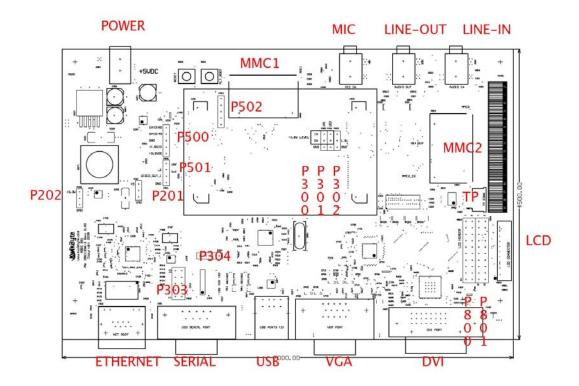
Figure 1-5: KBOC\_BB1 CONNECTOR/HEADER LABELS
